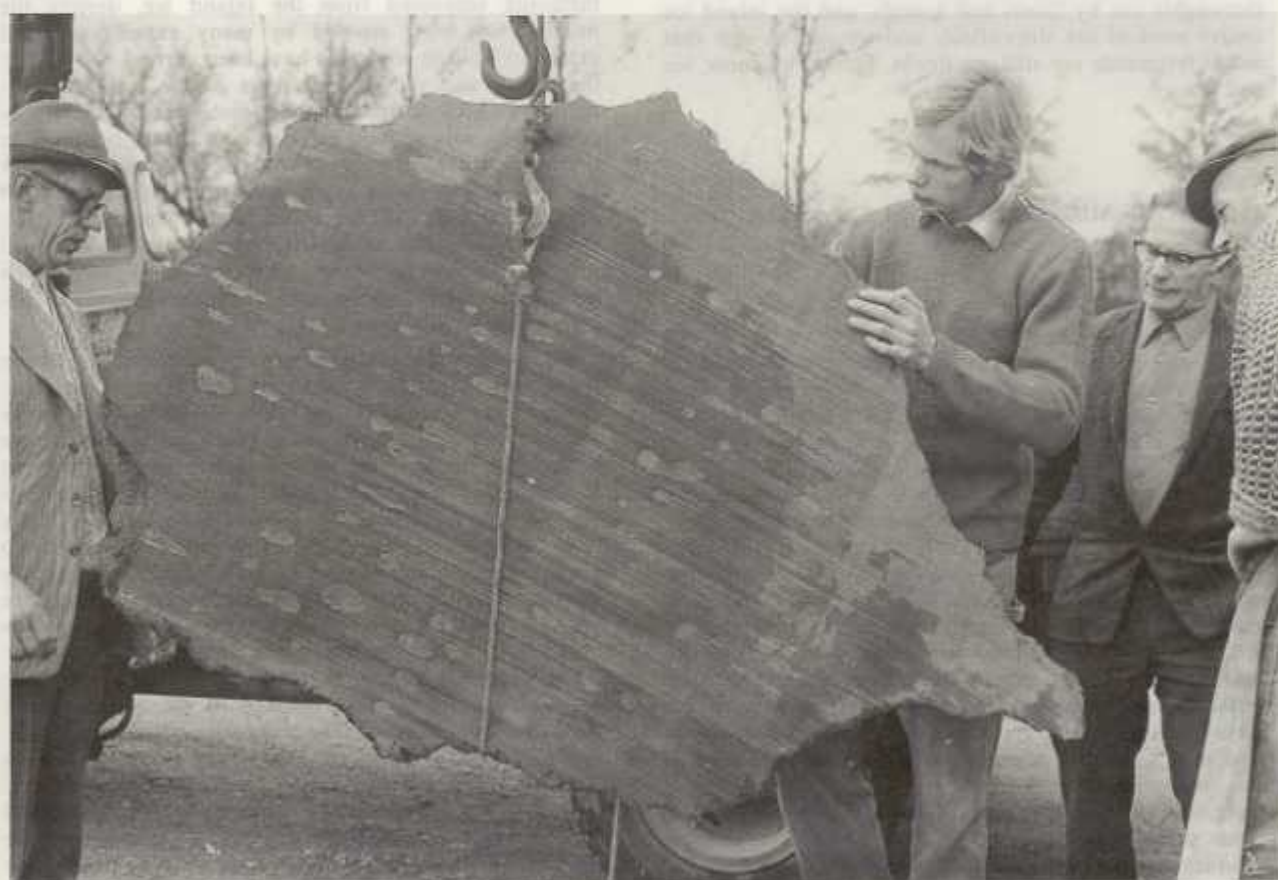
Fig. 12. In 1971 the Agpalilik meteorite was cut by the wire-saw technique. The large plate is 5 cm thick and weighs 560 kg. It was later polished and etched.
